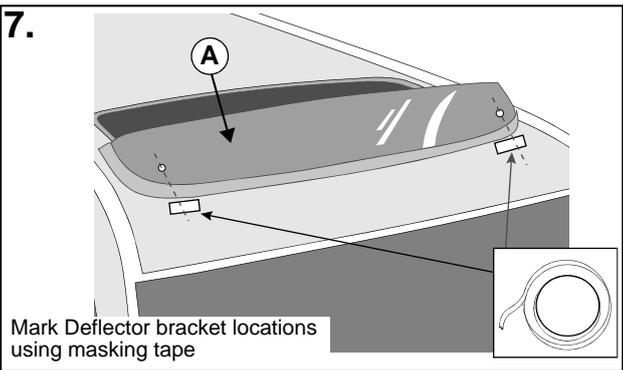
Mark Deflector bracket locations using masking tape
